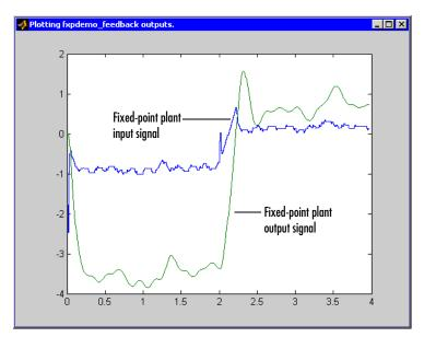
The Bode plot design sought to produce a well-behaved linear response for the closed-loop system. Clearly, the response is nonlinear. The nonlinear features are due to significant quantization effects. An important part of fixed-point design is finding scaling that reduce quantization effects to acceptable levels.
