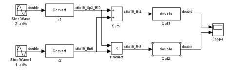
The model below displays its port data types:
