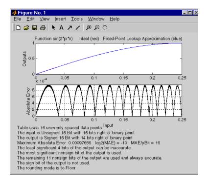
The upper plot shows the ideal function,  $\sin(2\pi x)$  and the fixed-point lookup approximation between the breakpoints. In this example, the ideal function and the approximation are so close together that the two graphs appear to coincide. The lower plot displays the errors.
