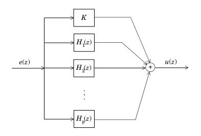
This expansion, where K is a constant and the  $H_i(z)$  are the first and second-order transfer functions, follows.
