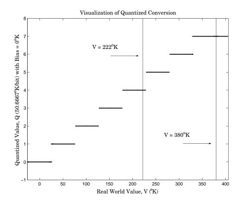
Notice that there are 7.5 possible quantization values. This is because only half of the first bit corresponds to temperatures (real-world values) greater than zero.
