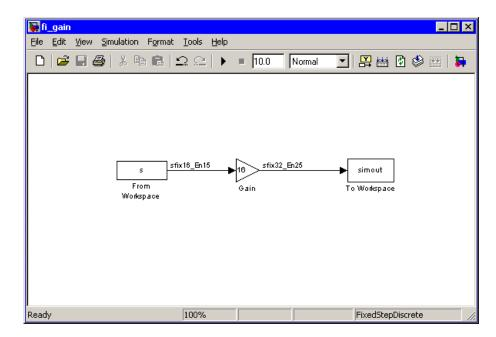
The To Workspace block writes the result of the simulation to the MATLAB workspace as a fi structure.
