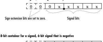
8-bit container for a signed, 6-bit signal that is positive or zero
