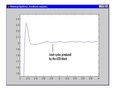
Note that a steady state has been achieved, but a small limit cycle is present in the steady state due to poor A/D design.
